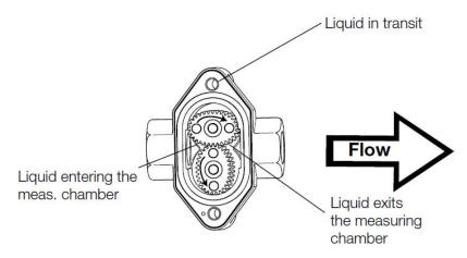
The positive displacement flow technology allows for precise flow measurement of most clean liquids regardless of the media conductivity. Other liquid properties also have a minimal effect on the performance of this type of meter. Flow profile conditioning and straight pipes run are not required as with other flow technology making oval gear installations simple to install in tight spaces and at an economical price.
