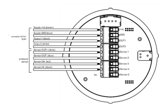
3. Depending on the desired configuration, the connection wires for output 1 (black wire) or output 2 (white wire) must now be removed from the terminals as shown in the illustration below.
