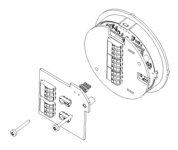
6. The free wire strands of the connector (5- or 8-pin) are now to be connected to the 2 connection terminals of the relay board as follows. In addition, the two slide switches must be brought into the correct position according to the arrows shown in the views.
