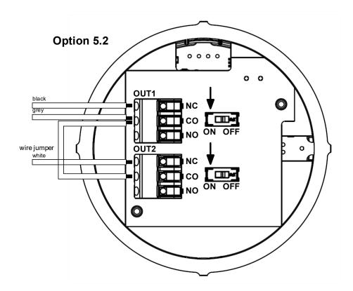
Note: To create a bridge between REL1 CO and REL2 CO, a 40 mm long piece must be cut from the gray wire, approx. 8 mm stripped on both sides and thus a bridge between the two CO terminals. For correct clamping, the individual conductors of both wire strands, which must be inserted in a terminal, must be twisted together before being inserted into the terminal.
