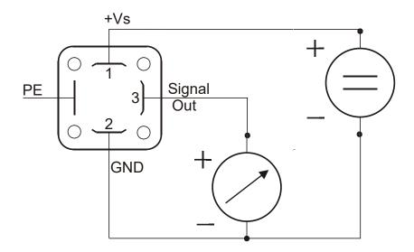
If the signal output is not used, the signal output (PIN 3) needs to be short-circuited with GND (PIN 2).
