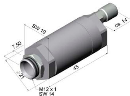
Air purge collar for TIN-SH combinable with mounting brackets Typ TIN-ZTAP2
