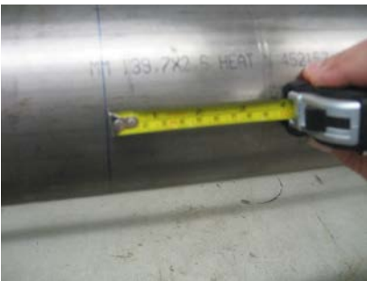
Figure 16: Mark the distance between transducer
