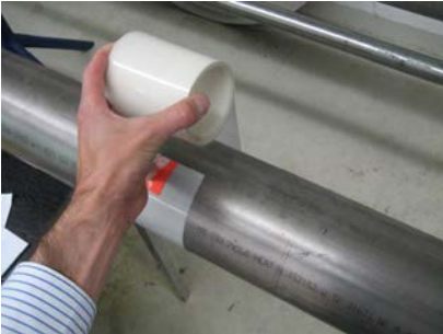
Figure 14: Attaching the template tape
