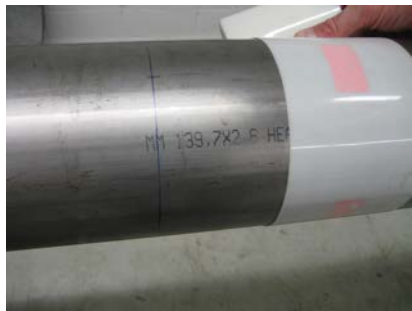
Figure 17: Mark the circumference for the second transducer.
