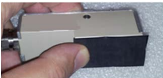
Figure 10: DUC-WF10 with acoustic coupling pad
