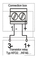
Connect limit value controller (+) brown cable (-) blue cable with transistor relay for devices without terminal box.
