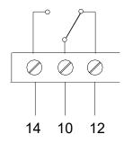
At all events it must be ensured when actuating loads such as contactors, relays etc. that the electrical limiting values are not exceeded – and not even briefly due, for instance, to voltage peaks. A contact protection relay is recommended to stop any contact overloading.
