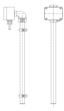
If present and not yet installed at the factory, fasten the transmitter to the bypass pipe with the tensioning straps and tighten it. The cable junction box is at the top. By default, the transmitter is mounted to the left of the standpipe. The transmitter must completely cover the two process connections.
