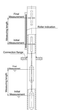
Remove the cotter pin from bottom end of the dip pipe, next, remove the transport lock of the float. Fix the float with the magnet system towards top and make sure, there are no remains of packing material or other impurities inside the tube.
