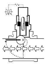
Media flowing in any direction moves the paddle, which rotates an eccentric, which in turn raises an assembly within the unit. The assembly has a permanent magnet mounted within it. This enables the magnet to activate a hermetically sealed reed switch. The signal from the reed switch can be used to trigger an alarm or indicator. With the appropriate relay, it is possible to automatically control pumps, motors or valves.
