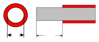
For power supply please use cables with a cross section of ca. 0.5...4 mm<sup>2</sup>. Solid cables should be dismantled about 8 mm to allow proper contact to terminals.
