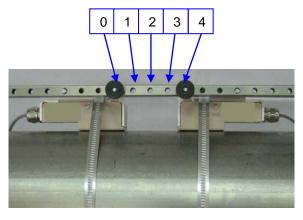
Picture 3 Example distance for bar index four using spacer bar for mounting
