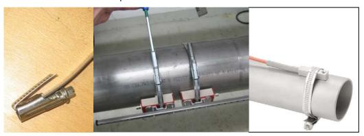
Pictures 7 Mounting DUC-WF Transducers, PT100 with stainless steel belts on a pipe
