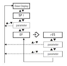
By pressing  $\triangle + \nabla$  simultaneously the menu will return to the base display or automatically after ca. 60 s without operation.
