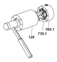
• Drive the screw set together with the bearing cover **080.1** out of the measuring housing **128** using light blows of a plastic hammer and pull out.
