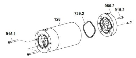
Remove the socket screws 915.1 and 915.2, take off the bearing cover 080.2. Remove the O- ring 739.2
