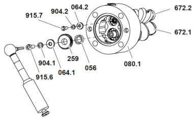
• Screw out the socket screw **915.6** with wedge lock washer **904.1** and supporting ring **064.1** at the measuring screw large **672.1**. Pull off the pole wheel **259** and distance ring **056**.
