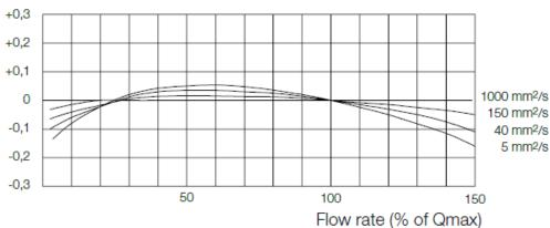
The measuring error refers to the actual flow rate. The diagram shows the characteristic for the OMS-... screw-type volumetric flow meter.
