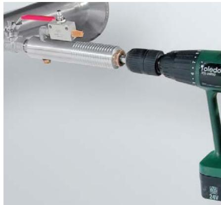
In case the system could not be shut down, means to be set depressurized, there could be used a spot drilling collar and drilling jig to drill through the ball valve.
