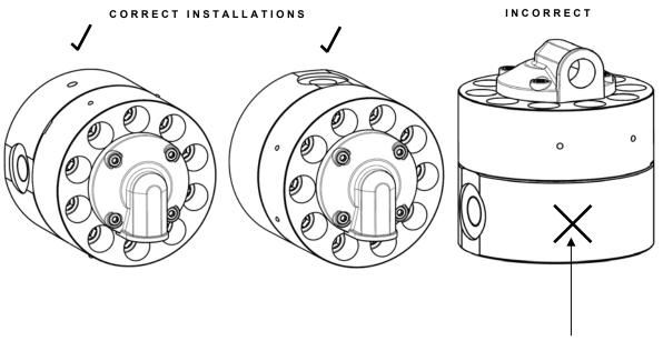
Incorrect installations will cause the rotor weight to be felt on the bottom of the measuring cavity.
