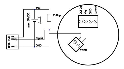
The individually specified maximum electrical values of the reed switch must never be exceeded, even for a moment. Higher switching values may reduce the service life or even destroy the contact.
