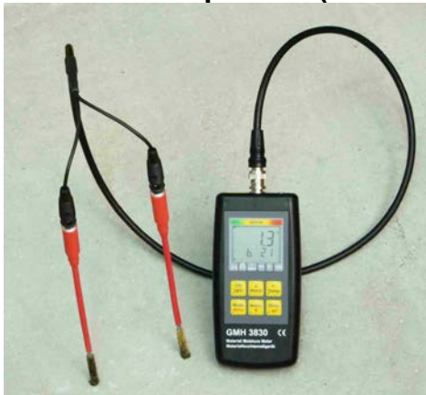
Measuring concrete with brush probe HND-FF06
