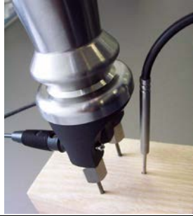
Reciprocating piston electrode HND-FF01 with temperature-probe –FF10
