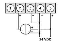
DAG-A3V in combination with a 3-wire-sensor 0-10 V
