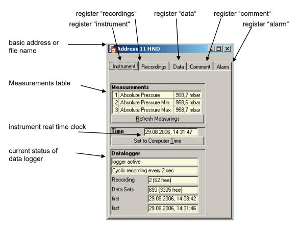
Please check real time clock and adjust it when necessary (by 'Set to Computer Time')
