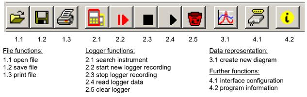
When moving the mouse pointer over a symbol a short description of the function is shown after a short time.
