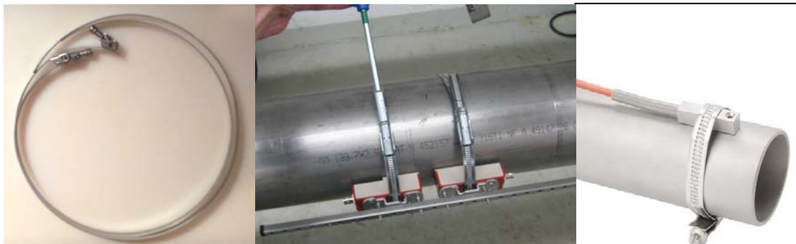
Pictures 10 Mounting US- Transducers, PT100 with stainless steel belts on a pipe
