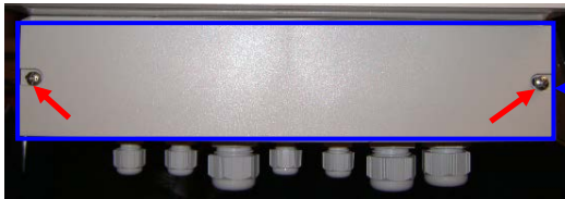
Picture 11 Removing cover plate from cable terminal
