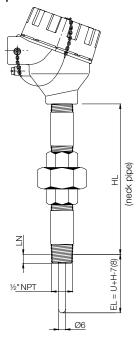
U = immersion length thermowell (see drawing thermowell)
