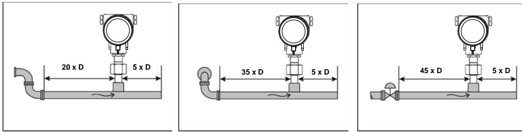
The values represent the min.lengths. In case the min. inlet / outlet runs could not be ensured, it must be expected to get increased or significant deviations of the measurement values.
