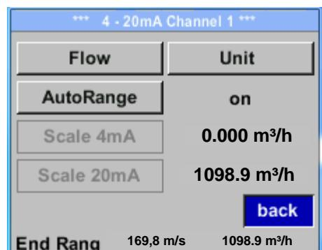
The 4-20 mA Analogue output of the Sensor KEC can be individually adjusted.
