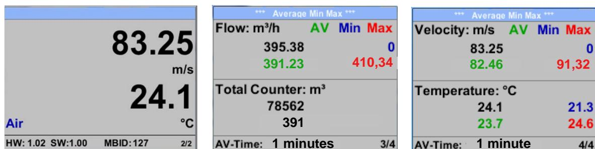
AV-Time (Period for average value calculation) could be changed under Sensor Setup.-Advanced– AV-Time
