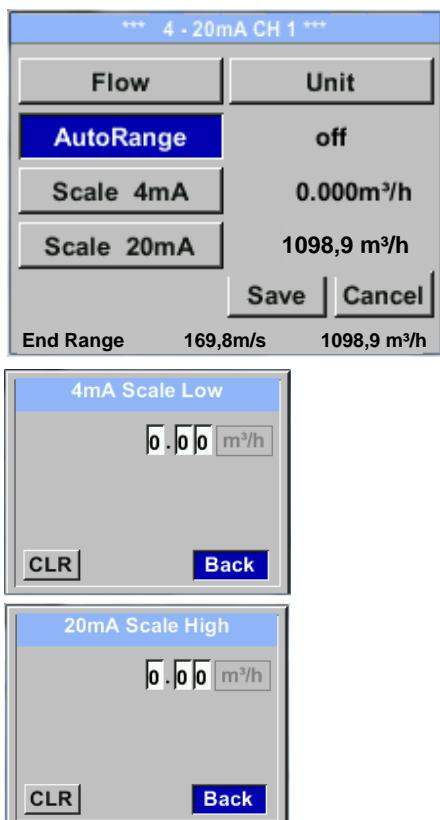
The scaling of the 4-20mA channel can be done automatically "Auto Range = on" or manual "AutoRange = off".
