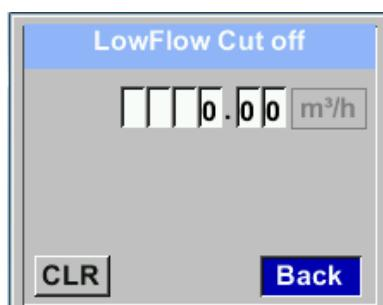
With the low-flow cut off activated, the flow below the defined "LowFlow Cut off" value will be displayed as 0 m<sup>3</sup>/h and not added to the consumption counter.
