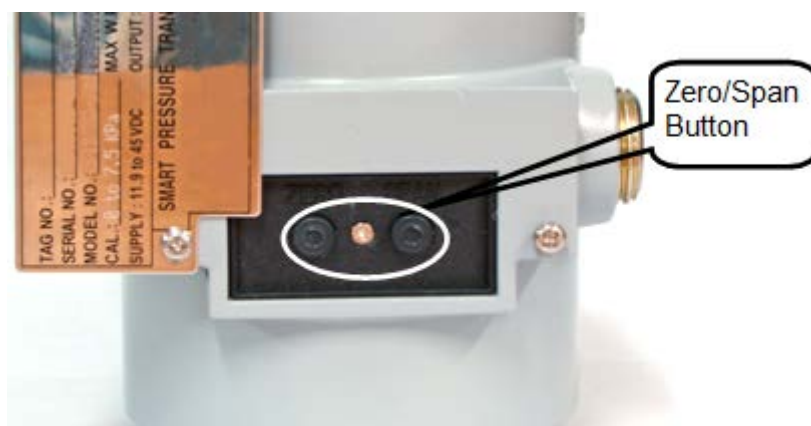
[Figure 4-4 Transmitter Zero/Span configuration Buttons]
