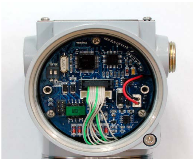
Figure 7.3 Structure of Electronics Module inner Transmitter
