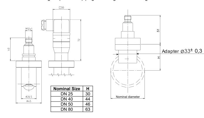
Position and weld-in the mounting adapter according to the nominal diameter suitable marking. The marking on the adapter must be in line with the outer diameter of the pipe. Also pay attention to the later position of the rotating vane (shaft of the vane shifted by 90° to the direction of flow).
