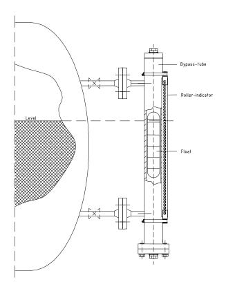
Remove bottom flange from bypass tube, and insert the cylindrical float in the NBK bypass tube with the designation "TOP" at the top. Reposition the gasket and close the bottom flange again; firmly tighten with screws.
