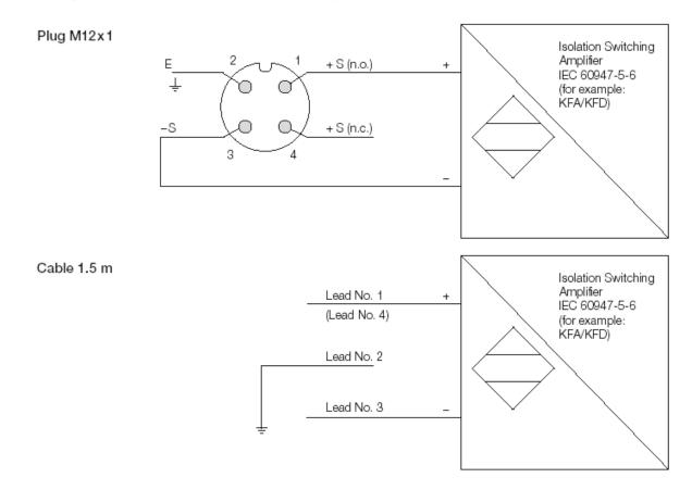
Wiring examples NWS-...2E... with Power supply unit acc. to IEC 60947-5-6
