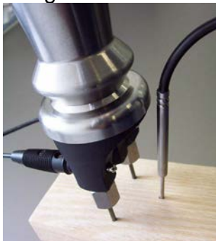
Reciprocating piston electrode HND-FF01 with temperature-probe HND-FF10
